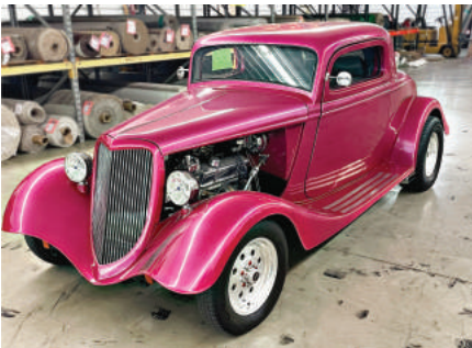
1934 Ford Coupe Kit Car from Street Beasts. Modified Chevy 350 engine, 350 turbo transmission, Mustang II frame.
