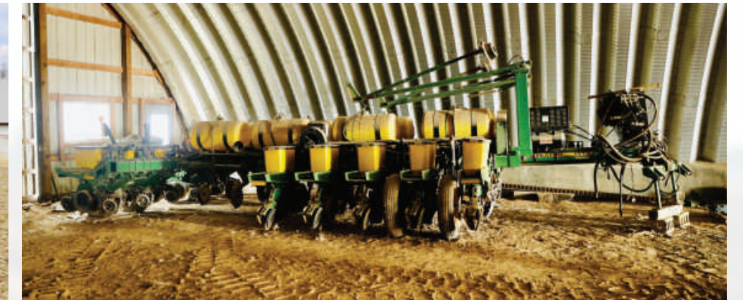
11.) JD 1770 planter, hydraulic air compressor , up/down, auto row shutoff, 2 vacuum motors
