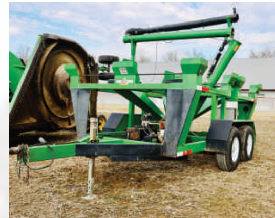
10.) JD seed cart, self-contained hydraulics, holds 4 seed boxes, electric brakes, liquid seed treater on back
